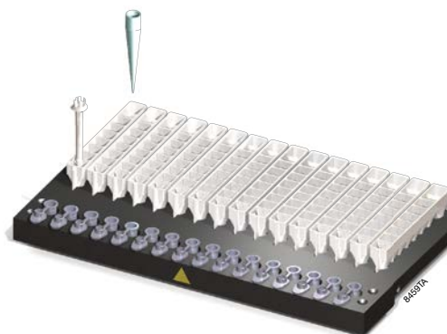
Figure 3. The LEV plunger is placed in well #8 of the cartridge (the well closest to the Elution Tube), and lysates are placed into well #1 of the cartridge.
