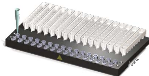
Figure 2. The Elution Tubes are placed in the front of the Maxwell® 16 LEV Cartridge Rack, and 50µl of Nuclease-Free Water is dispensed into each tube.
