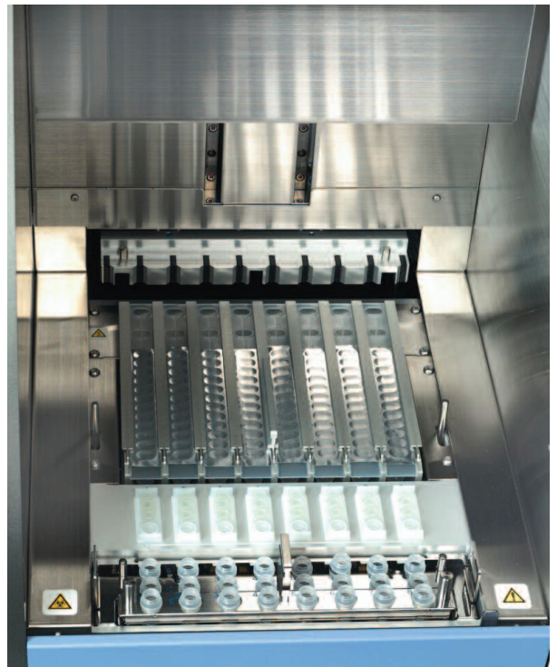
▲ Figure 5: Pipetting station and nozzle head. During the isolation process, a stepper motor moves the cartridge stage holding the Reagent Cartridges and the Sample and Elution tubes. An eight-nozzle pipetting head processes the samples, from piercing the sealing foil on the cartridge to the final nucleic acid elution. A pressure sensor integrated into the nozzle head detects accidental clotting or tip loss during sample processing.
