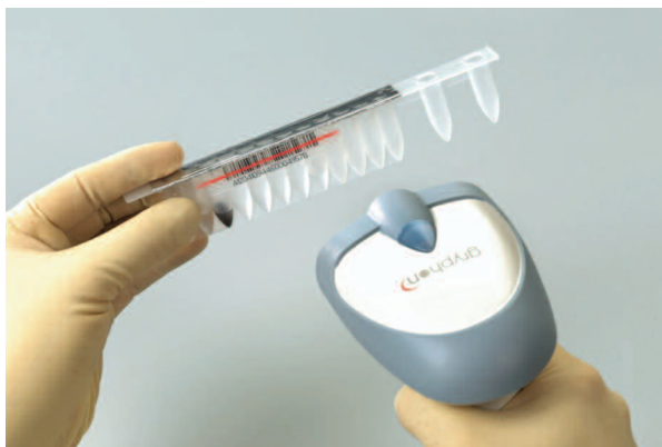
▲ Figure 7: Kit information in the Reagent Cartridge barcode. Each kit's Reagent Cartridges are labeled with a barcode with information about kit name, lot, and expiration date. Based on this information, the MagNA Pure Compact software selects appropriate protocols and notifies the user if the kit is expired. All barcode data are automatically saved by the system.
