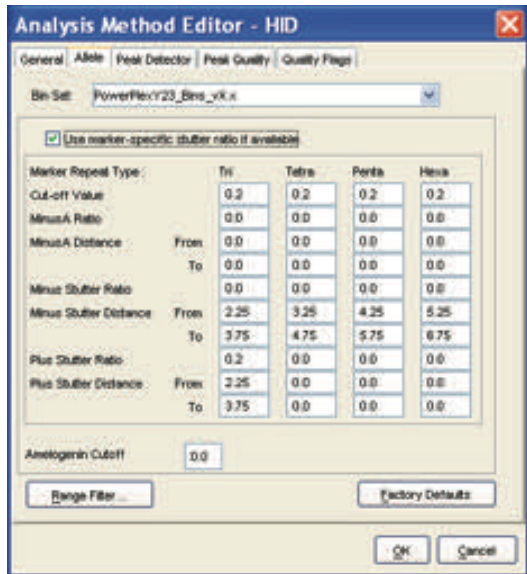
Figure 21. The GeneMapper® ID Software Allele tab with settings for using a 20% peak filter.
