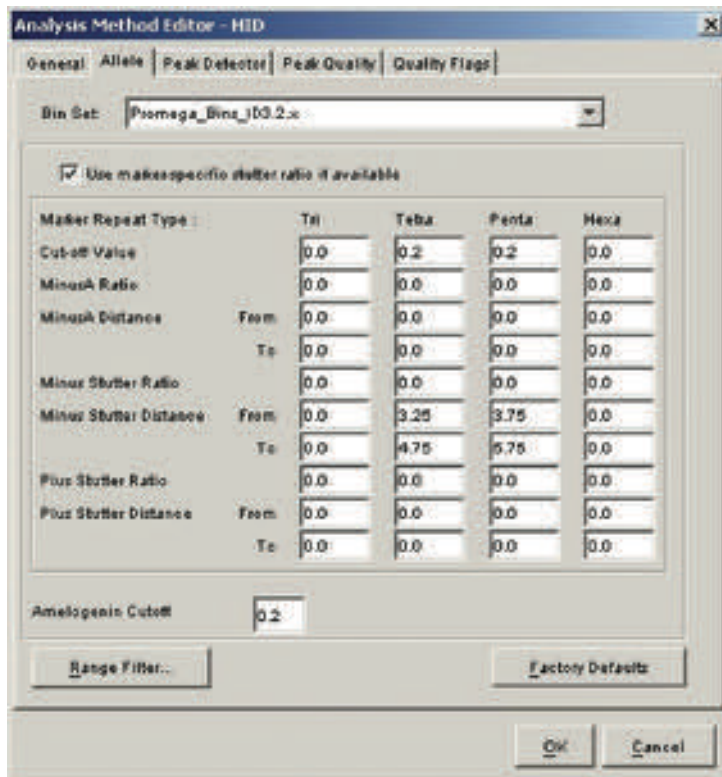
Figure 22. The GeneMapper® ID Allele tab with settings for using a 20% peak filter.
