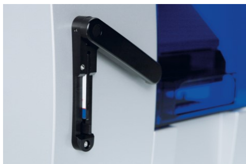
Figure 3. Complete insertion of EZ1 Card. The EZ1 Card must be completely inserted before the EZ1 instrument is switched on.
