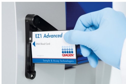
Figure 2. Ease of protocol setup using EZ1 Cards. Inserting an EZ1 Card that contains protocol into an EZ1 instrument. The instrument should only be switched on after an EZ1 Card is inserted. EZ1 Cards should not be exchanged while the instrument is switched on.
