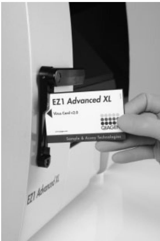
Figure 1. Ease of protocol setup using EZ1 Cards. Inserting an EZ1 Card, containing a protocol, into an EZ1 instrument. The instrument should only be switched on after an EZ1 Card is inserted. EZ1 Cards should not be exchanged while the instrument is switched on.
