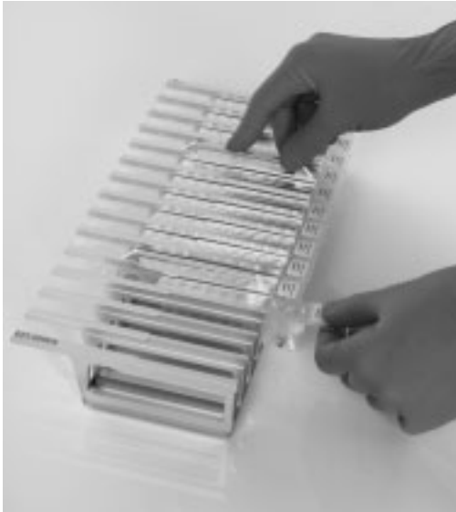
Figure 3. Ease of setup using reagent cartridges. A A sealed, prefilled reagent cartridge. Fill levels vary, depending on the type of reagent cartridge. B Loading reagent cartridges into the cartridge rack. The cartridge rack itself is labeled with an arrow to indicate the direction in which reagent cartridges must be loaded.
