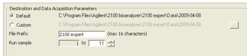
Data will be saved automatically to a file with a name using the prefix you have just entered. At this time you can also customize the file storage location and the number of samples that will be analyzed.
