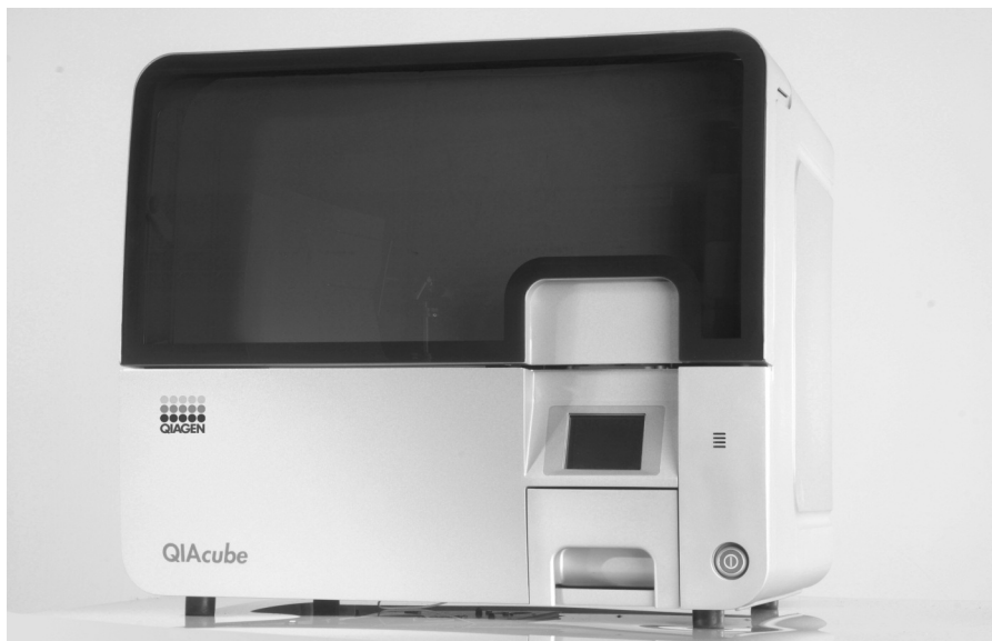
Figure 1. Automated viral RNA purification. Viral RNA purification using the QIAamp Viral RNA Mini Kit can be fully automated on the QIAcube.
