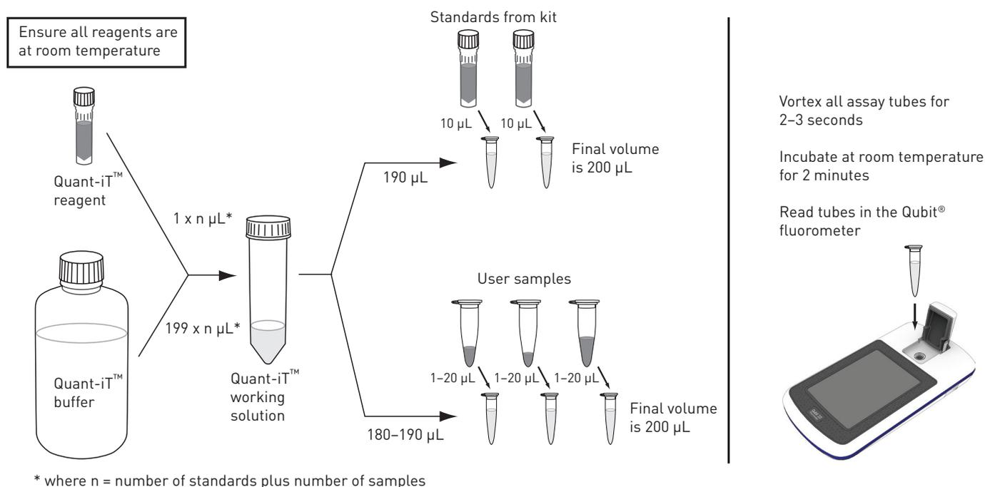
Figure 4. Overview for using the Quant-iT™ RNA assay in the Qubit® fluorometer.
